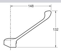
Product Specification: Elbow-control lever. E18164. Collection: EASY. MATERIAL: Metal. Long elbow-operated lever.
