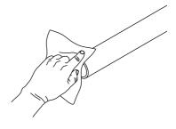
Remove the burr inside and outside. Clean pipe inside diameter using residue-free silicone and oil-free cleaning products (e.g. methylated spirits).
