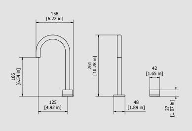
Cartridge Threaded fitting G1/2" female 400mms Ø25 progressive cartridge Aerator Flow Rate (+/-10%) 1 BAR 2 BAR 3 BAR M16.5x1 3 I\m 3.8 l\m 3.8 l\m
