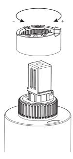
Turn the temperature limiting ring clockwise (+) to increase maximum hot temperature, anti-clockwise (-) to reduce the maximum hot temperature.
