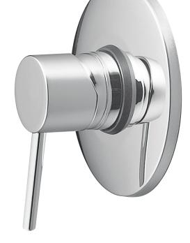
CONSTRUCTION: Brass body CARTRIDGE TYPE: Ceramic with Fastflow II technology CLASSIFICATION: Suitable for all pressure systems CONNECTIONS: 1/2 " BSP Male WORKING PRESSURE UNEQUAL COLD: 17 - 120kPa WORKING PRESSURE UNEQUAL HOT: 300 - 500kPa (If supply exceeds 500kPa a pressure limiting valve must be installed) DIMENSIONS FOR FITTING: Ø100mm hole OPERATING TEMPERATURE: 5 °C - 80 °C
