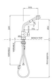
CONSTRUCTION: Brass body CARTRIDGE TYPE: SP033510 ceramic cartridge CLASSIFICATION: Suitable for mains pressure only INLET CONNECTIONS: 1/2 " BSP Female WORKING PRESSURE: 150 - 1000kPa DIMENSIONS FOR FITTING: 40mm diameter hole OPERATING TEMPERATURE: 5 °C - 80 °C WATER FLOW RATE: mains pressure (7.0 l/pm)
