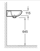
Product Specification: Handwash basin 45 cm. E4338. Collection: BRIVE. DIMENSIONS: 45 x 35 cm. WEIGHT: 8.2 kg. MATERIAL: Ceramic. INSTALLATION TYPE: Self-supporting. FAUCET DRILLING: 1 tap hole. FIXINGS: Bolts. TAP DRILLING: 1 tap hole. INSTALLATION: STANDARD. OVERFLOW: With overflow hole. PRODUCT INCLUDED: (Tap not included). Functional design with backsplash.
