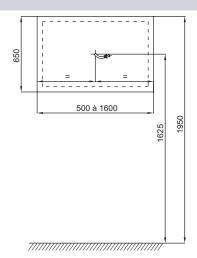
Product Specification: Mirror 60 cm - edge lighting and anti-steam feature. EB1440. Collection: NO COLLECTION. DIMENSIONS: 60 x 4.30 x 65 cm. WEIGHT: 7 kg. MATERIAL: Glass. INSTALLATION TYPE: Wall-mount. POWER: 230V, 10W, class II, IP 44. ANTI-STEAM: Yes. TEMPERATURE: 4000° K.
