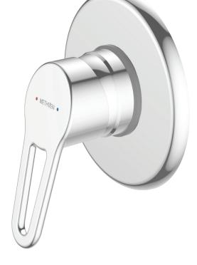
CONSTRUCTION: Brass body CARTRIDGE TYPE: Ceramic with Fastflow II technology CLASSIFICATION: Suitable for all pressure systems CONNECTIONS: 1/2 " BSP Male WORKING PRESSURE UNEQUAL COLD: 17 - 120kPa WORKING PRESSURE UNEQUAL HOT: 300 - 500kPa (If supply exceeds 500kPa a pressure limiting valve must be installed) DIMENSIONS FOR FITTING: Ø100mm hole OPERATING TEMPERATURE: 5 °C - 80 °C
