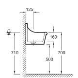
Product Specification: Wall-hung slop sink. E1898. Collection: NORMA. DIMENSIONS: 45 x 35 cm. WEIGHT: 14.2 kg. MATERIAL: Ceramic. INSTALLATION TYPE: Self-supporting. Undrilled version.
