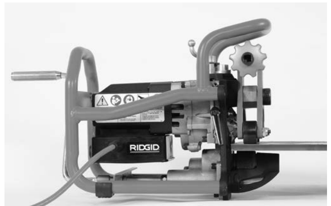
Figure 16B – Installing Beveller on Plate
