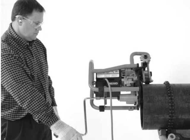
Figure 20A – Bevelling Operation (Fixed Workpiece/Moving Beveller)
