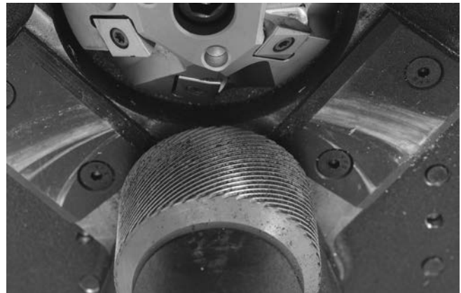
Figure 22– Clean Drive Roll Knurls
