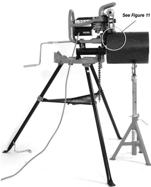
Figure 12 – Fixed Beveller, Short Pipe, One Pipe Stand
