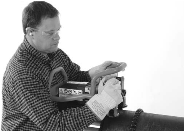
Figure 17A – Hand Tighten Clamp Screw
