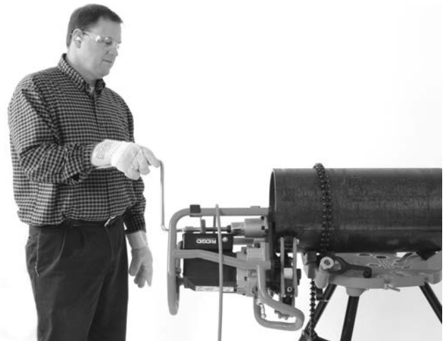
Figure 20B – Bevelling Operation (Fixed Workpiece/Moving Beveller)
