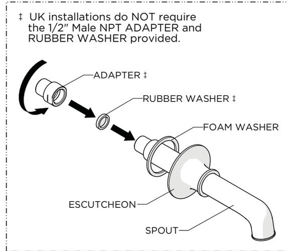
‡ UK installations do NOT require the 1/2" Male NPT ADAPTER and RUBBER WASHER provided.
