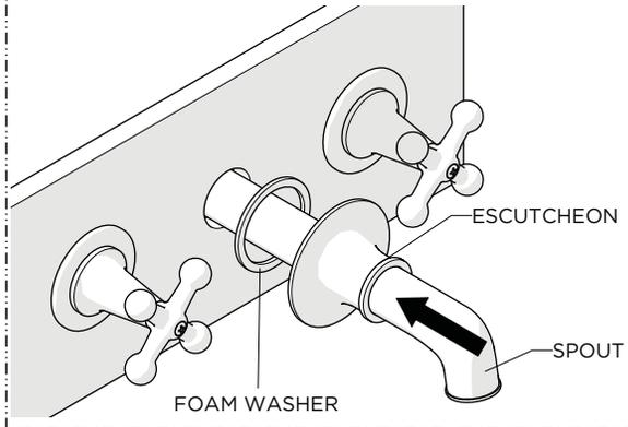
22. Slide the ESCUTCHEON against the finished wall making sure to use the FOAM WASHER provided.
