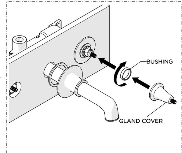
12. Thread the PLASTIC BUSHING onto the TRIM NUT then place the GLAND COVER over the TRIM NUT making sure it is fully seated.
