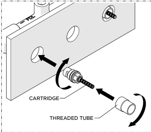
7. Repeat Steps 2 - 6 to cut the second [2<sup>nd</sup>] THREADED TUBE and CARTRIDGE STEM.
