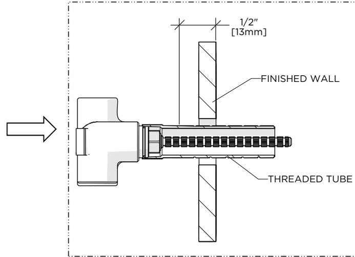
2. Mark the THREADED TUBE 1/2" [13mm] behind the finished wall.
