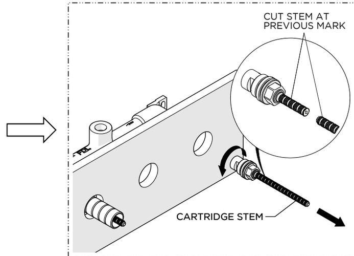
5. Remove the CARTRIDGE using a 21/32" [17mm] shower valve socket wrench (not provided) then cut the STEM at the previous mark.
