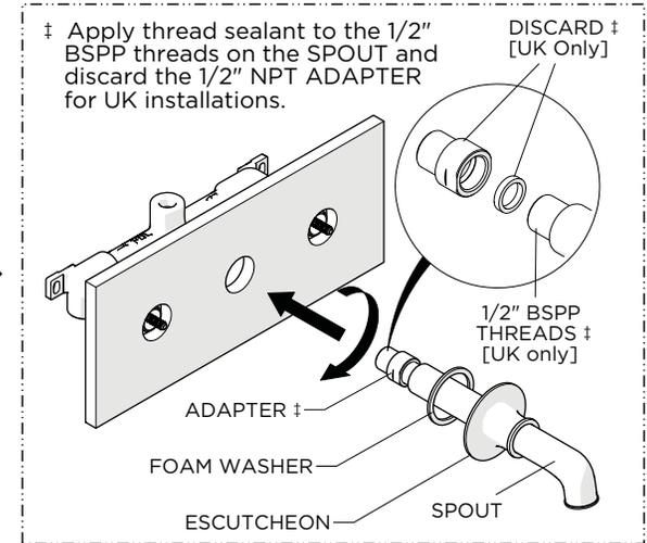
‡ Apply thread sealant to the 1/2" BSPB threads on the SPOUT and discard the 1/2" NPT ADAPTER for UK installations.
