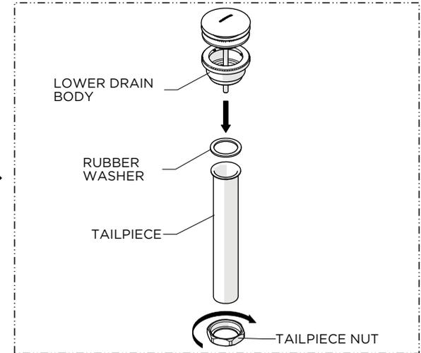
15. Remove the **TAILPIECE** from the **LOWER DRAIN BODY**.
