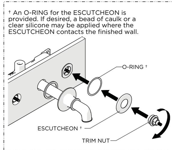
‡ An O-RING for the ESCUTCHEON is provided. If desired, a bead of caulk or a clear silicone may be applied where the ESCUTCHEON contacts the finished wall.
