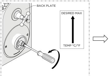
19. With water running, rotate the SQUARE TUBE to adjust the temperature to the maximum desired bathing temperature, verified with a thermometer. Turn the water off and make sure not to change this setting.
