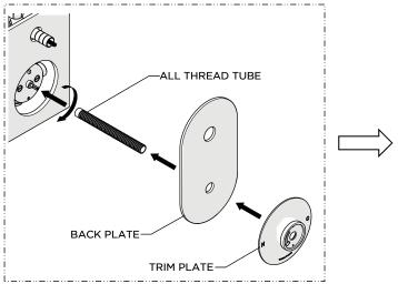
Thread the ALL THREAD TUBE onto the THERMOSTATIC CARTRIDGE then slide the BACK PLATE and TRIM PLAET over the TUBE.
