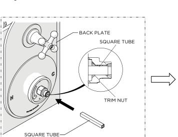
16. Re-insert the SQUARE TUBE back into the TRIM NUT making sure it is slight recessed.
