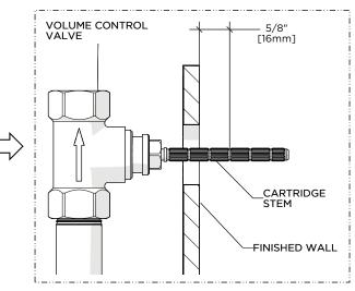
Mark the VOLUME CONTROL CARTRIDGE STEM 5/8" [16mm] beyond where it protrudes from the finished wall.
