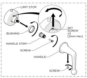
20. Loosen the FINISHED SCREW, remove the HANDLE, unthread the PLASTIC BUSHING to expose the SET SCREWS and loosen them using a 2mm hex key. It is **NOT** necessary to remove the HANDLE STEM.
