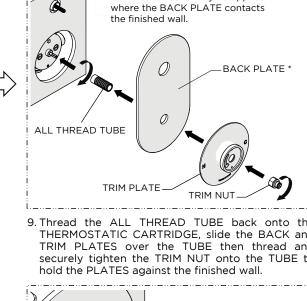
9. Thread the ALL THREAD TUBE back onto the THERMOSTATIC CARTRIDGE, slide the BACK and TRIM PLATES over the TUBE then thread and securely tighten the TRIM NUT onto the TUBE to
