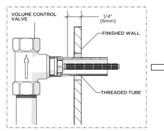
4. Mark the THREADED TUBE 1/4" [6mm] behind the finished wall.
