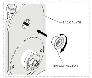
and securely tighten the CONNECTOR onto the THREADED TUBE.
