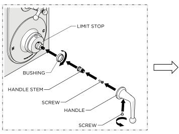
23. Thread the BUSHING back onto the LIMIT STOP, making sure the HANDLE STEM is securely attached to the LIMIT STOP, place the HANDLE onto the HANDLE STEM and over the BUSHING in the desired orientation, then thread and securely tighten the FINISHED SCREW.
