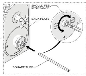
14. Insert the SQUARE TUBE into the TRIM NUT then, by feel, make sure it slides over the CARTRIDGE STEM and is fully seated.
