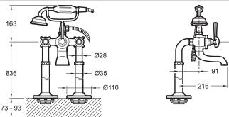
Product Specification: Floor-mount mixer. E24314. Collection: CLÉO 1889. DIMENSIONS: 26 x 125 cm. WEIGHT: 8.1 kg. MATERIAL: Metal. INSTALLATION TYPE: Floor-mount. TYPE: Mixer. CONNECTION: With supply hoses. MECHANISM GUARANTEE: 5 years. FINISH GUARANTEE: Chrome 10 years / PVD 25 years.
