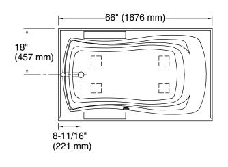
No change in measurements if connected with drain illustrated. (K-7161-AF) Recommended Faucet Location
