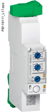
IFM Modbus communication interface. Ref.: LV434000.
