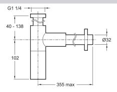
Product Specification: Design bottle trap, long version. E78291. Collection: NO COLLECTION. WEIGHT: 1 kg. MATERIAL: Metal. INSTALLATION TYPE: Wall-mount.
