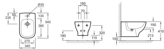
Product Specification: Wall-hung bidet. EMC0001. Collection: STRUKTURA. DIMENSIONS: 54 x 34 cm. WEIGHT: 19 kg. MATERIAL: Ceramic. INSTALLATION TYPE: Wall-hung. HEIGHT: Standard. PRODUCT INCLUDED: (Tap not included). 1 tap hole.
