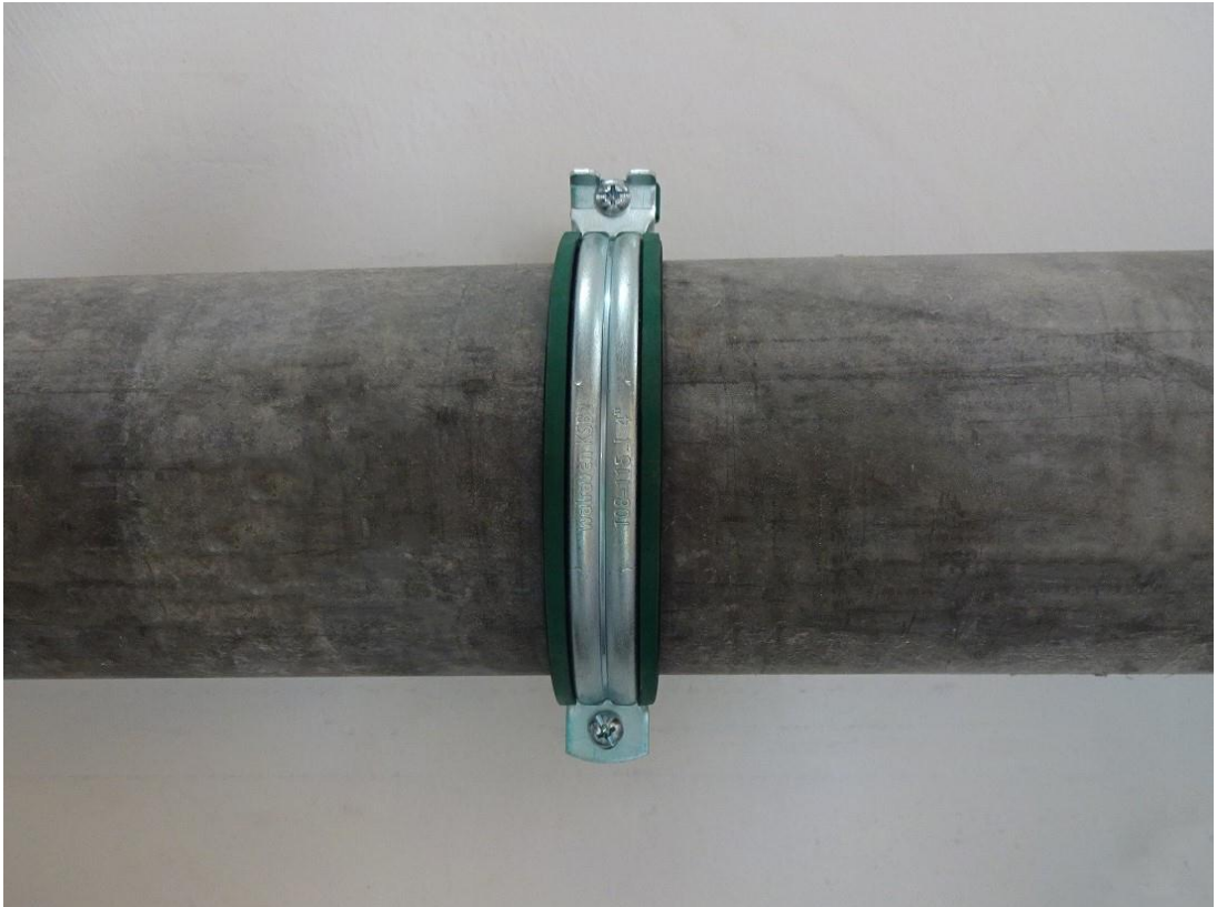
Fig. 2: Meas. 4: KSB2 two-screw-clamp, 4" (108 - 115 mm), connection M8/10, with EPDM-rubber (23 x 4,20 mm)
