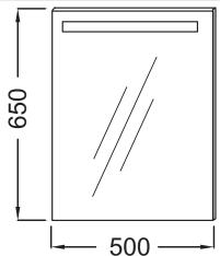
Product Specification: Mirror 50 cm - LED lighting and anti-steam feature. EB1410. Collection: NO COLLECTION. DIMENSIONS: 50 x 3 x 65 cm. WEIGHT: 7 kg. MATERIAL: Glass. INSTALLATION TYPE: Wall-mount. POWER: 230V, 17W, class II, IP 44. ANTI-STEAM: Yes. infrared sensor switch located below the mirror.
