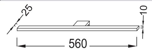
Product Specification: "Eclat" LED spotlight. EB1237. Collection: NO COLLECTION. DIMENSIONS: 56 x 2.50 x 1 cm. WEIGHT: 0.4 kg. MATERIAL: Metal. INSTALLATION TYPE: Wall-mount. POWER: 230V, 7W, Class II IP44. TEMPERATURE: 4000°K.
