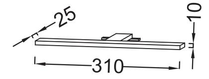
Product Specification: "Aube" LED spotlight. EB1224. Collection: NO COLLECTION. DIMENSIONS: 31 x 2.50 x 1 cm. WEIGHT: 1 kg. MATERIAL: Metal. INSTALLATION TYPE: Wall-mount. POWER: 230V, 3.5W, class II IP 44. TEMPERATURE: 4000°K.
