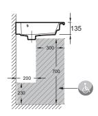
Product Specification: Vanity top 120 cm. EXAT112. Collection: ODÉON RIVE GAUCHE. DIMENSIONS: 121 x 51.20 cm. WEIGHT: 35.1 kg. MATERIAL: Ceramic. INSTALLATION TYPE: Self-supporting. TAP DRILL-ING: 2 tap holes. GROUND/UNGROUND: Without ground underside. OVERFLOW: With.
