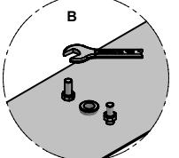
Screw the screws of the cover starting from the base of the shower arm.
