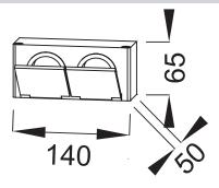
Product Specification: Electrical outlet. EB1555. Collection: ODÉON RIVE GAUCHE. DIMENSIONS: 14 x 5 x 6.50 cm. WEIGHT: 0.4 kg. MATERIAL: Plastic. STORAGE: Accessoires pour meuble. POWER: 220V. INSIDE FINISH: Black.
