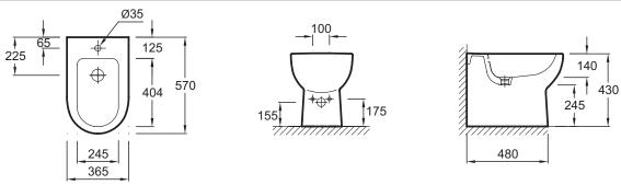
Product Specification: Bidet. E4738. Collection: ODÉON UP. DIMENSIONS: 57 x 36.50 cm. WEIGHT: 22.6 kg. MATERIAL: Ceramic. INSTALLATION TYPE: Floor-standing. HEIGHT: Comfort. RIM TYPE: Open (tradi-tional). 1 tap hole.
