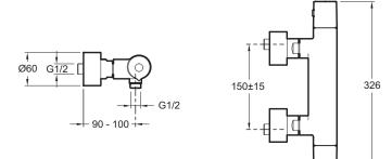
Product Specification: Thermostatic single-lever wall-mount shower mixer. E97384. Collection: AVID. WEIGHT: 3.5 kg. MATERIAL: Brass. INSTALLATION TYPE: 2 holes. NORMS AND REGULATION: ACS : 14 ACC LY 587. TYPE: Single-lever. FLOW RATE: 13 I/mn. CONNECTION: With connectors and wall escutcheons. HOLE CONFIGURATION: 150 ± 15. SAFETY STOP: 40°C. MECHANISM GUARANTEE: 5 years. Non-return valves on supplies.
