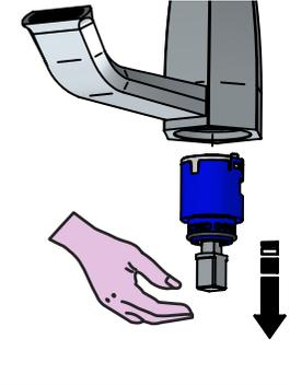
**SOSTITUZIONE AERATORE / AERATOR REPLACEMENT**
