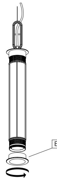
**EN** Unscrew the base cap (E) from the main body of the lamp module.
