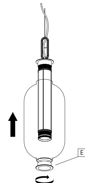
**EN** Position the glass diffuser over the main body of the lamp module, and then re-fasten the base cap (E) to hold it in place.
