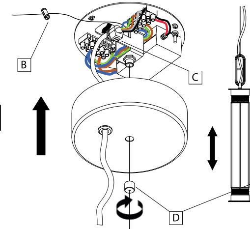
**EN** Hang the lamp module by the steel wire suspension cable as shown in the diagram, and adjust to desired height using clamp (B). Secure the electrical cable to the lamp using clamp (C). Fit the rose cap and secure it with the knurled screw (D).
