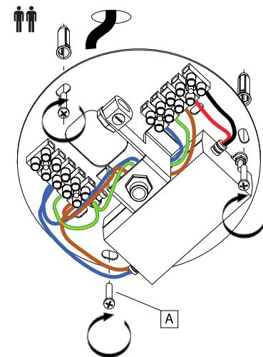
**EN** Drill holes in the ceiling positioned according to the template of the ceiling rose and install the screw anchors. Fix the ceiling rose into the ceiling with screws (A).
