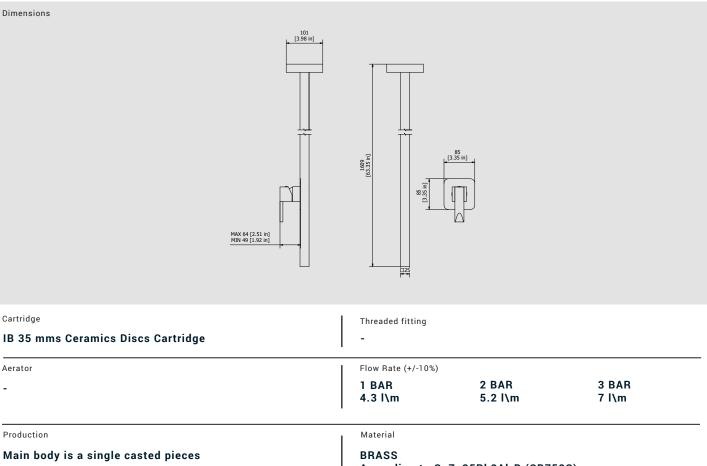
According to CuZn35Pb2AI-B (CB752S) Max Lead content: 1.36%
