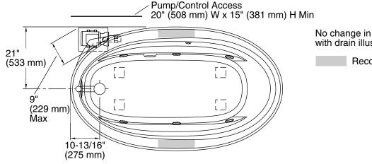
No change in measurements if connected with drain illustrated. (K-11677)
