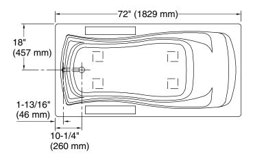
No change in measurements if connected with drain illustrated. (K-7166-AF) Recommended Faucet Location
