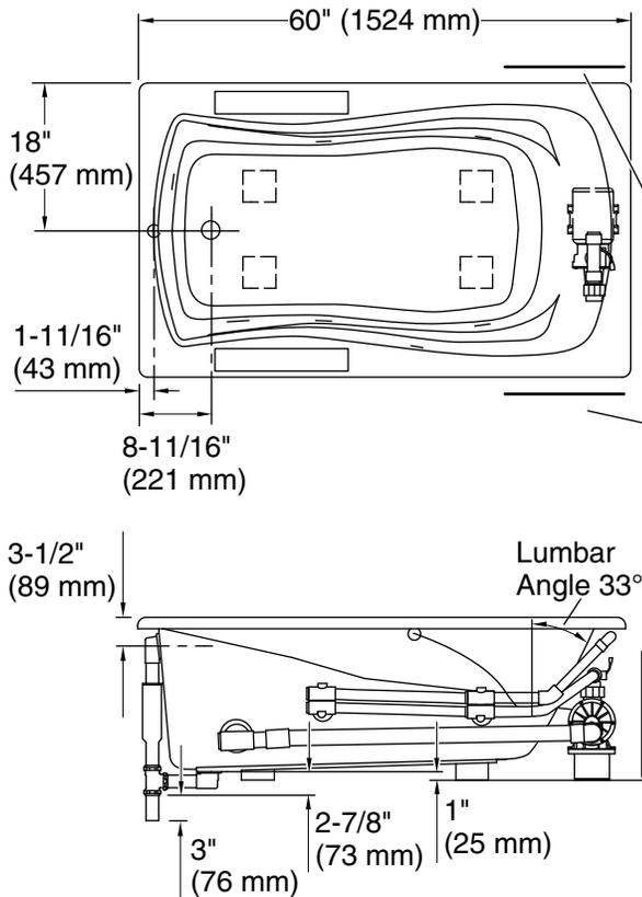
No change in measurements if connected with drain illustrated. (K-7161-AF)
