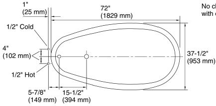
No change in measurements if connected with drain illustrated. (K-106)
