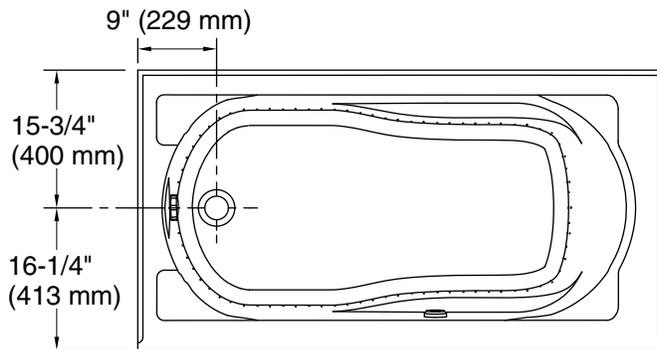
No change in measurements if connected with drain illustrated. (K-7213)
