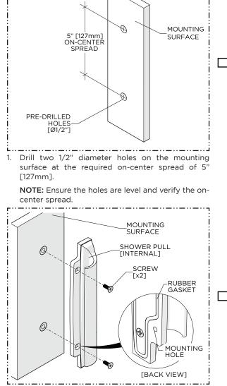
3. Hold the internal SHOWER PULL up to the mounting surface and align the mounting holes then insert the SCREWS provided.
