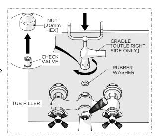
Using the RUBBER WASHER provided and with the outlet to the right, thread and securely tighten the HANDSHOWER CRADLE onto the TUB FILLER.
