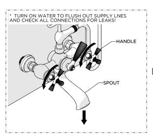
4. Turn on the water to flush out the supply lines and check all connections for leaks.
