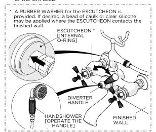
With water running, operate the DIVERTER HANDLE to ensure it and the HANDSHOWER function properly.
