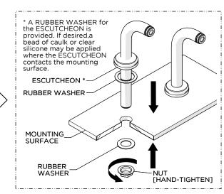
Making sure the RUBBER WASHER provided is beneath the ESCUTHCEON, insert each UNION through the hole on the mounting surface then reinstall the MOUNTING HARDWARE and handtighten the NUT.
