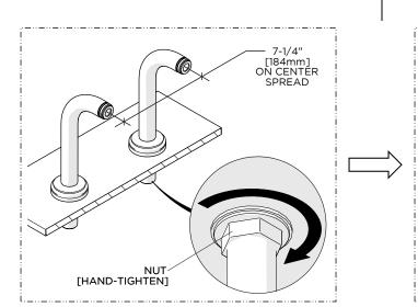
3. Verify the UNIONS are level, parallel to each other, and at the proper 7-1/4" [184mm] on-center spread then securely tighten the NUTS.
