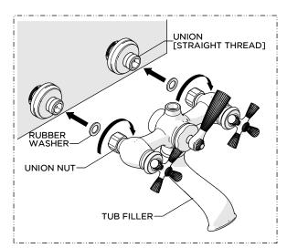
Using the RUBBER WASHERS provided, hold the TUB FILLER up to the UNIONS then thread and securely tighten the NUTS onto the UNIONS.
