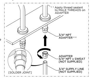
4. Apply thread sealant to the male threads on each NPT ADAPTER then thread and securely tighten 3/4" NPT x SWEAT ADAPTERS (NOT SUPPLIED). Adjust the length of each supply line as needed and complete final connections then PORCEED TO THE TUB FILLER INSTALLATION SECTION.
