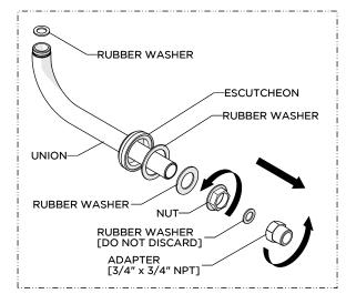
Remove the ADAPTER and MOUNTING HARDWARE from each UNION, NOTE: Do NOT remove the RUBBER WASHER beneath the ESCUTCHEON or discard the 3/4" RUBBER WASHERS provided.
