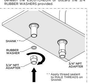
4. Apply thread sealant to the male threads on each SHANK then thread and securely tighten the NPT ADAPTERS onto them, making sure to use the RUBBER WASHERS provided.
