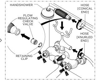
3. Thread the conical end of the HOSE to the HANDSHOWER and the other end to the CRADLE then rest the HANDSHOWER on the CRADLE
