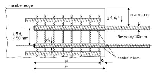
$^{1)}$  If the clear distance between lapped bars exceeds  $4d_s$  then the lap length shall be increased by the difference between the clear bar distance and  $4d_s$
