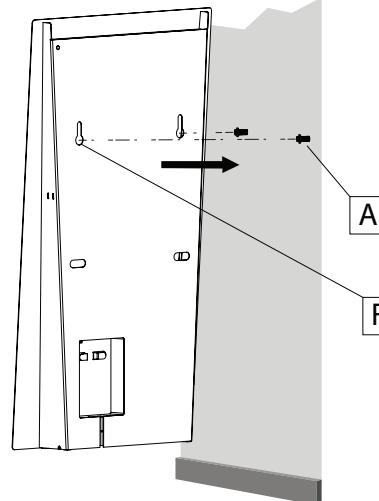
EN 4.1 To fix the lamp, position the holes (F) with the anchors supplied .
