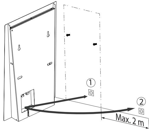
EN To carry out the installation, you must choose between installation (1) or (2) depending on the position of the power socket.
