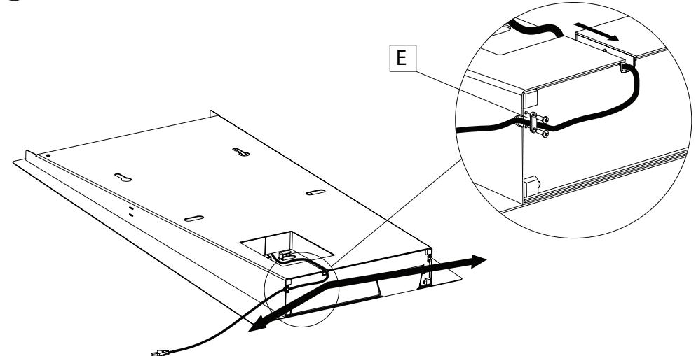
EN If installation (2) is chosen, the electric cable must be passed through the groove and fixed firmly with the cable gland (D) on the right or left depending on the position of the power socket.
