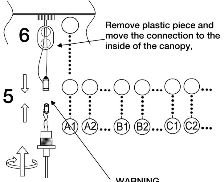
Remove plastic piece and move the connection to the inside of the canopy,
