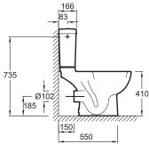
Product Specification: WC pan, P-trap. 4956CK. Collection: ODÉON UP. DIMENSIONS: 67 x 36.50 cm. WEIGHT: 23.5 kg. MATERIAL: Ceramic. INSTALLATION TYPE: Floor-standing. VOLUME OF WATER: 2.6/4 L and 3/6 L. HEIGHT: Comfort. RIM TYPE: Open (traditional). RIM: With rim. PRODUCT INCLUDED: (Cistern and seat not included). WATER USE: Water-efficient 2.6/4 L dual flush or 3/6 L standard flush. P-trap. Cistern not included.
