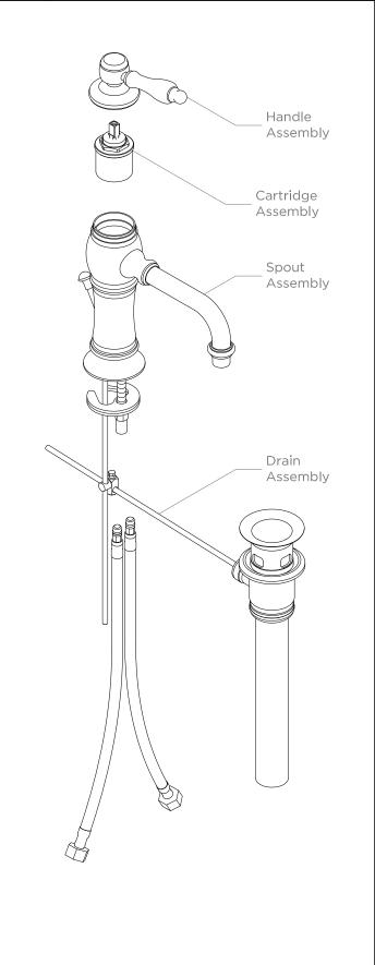
These guidelines have been prepared for the professional contractor to aid in the installation of: <a href="JULIA BRIDGE">JULIA BRIDGE ONE HOLE DECK MOUNTED LAVATORY FAUCET WITH METAL LEVER HANDLE(JULSO9)</a>. All dimensions are based on origin specification and are subject to change and variation. Please consult your Design Associate for current specifications.
