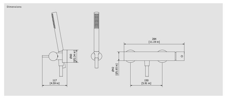
Cartridge Treaded fitting G1/2" male Ø35 ceramic cartridge
