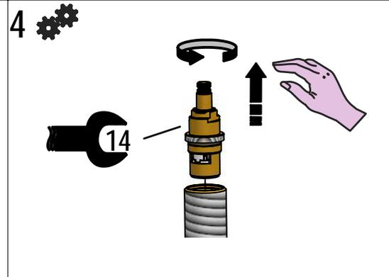
**! SOSTITUZIONE SNODINO BIDET/ JOINT BIDET REPLACEMENT**
