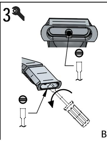
**! SOSTITUZIONE AERATORE / AERATOR REPLACEMENT**
