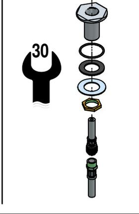
**! SOSTITUZIONE AERATORE / AERATOR REPLACEMENT**
