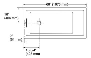
No change in measurement if connected with drain illustrated. (K-7272)
