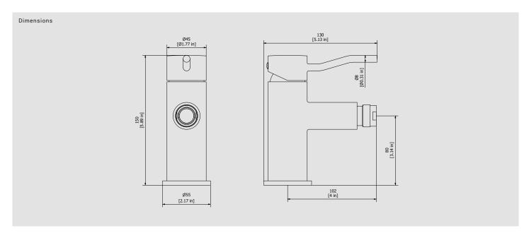
Cartridge Threaded fitting G3/8" female Ø35 ceramic cartridge Aerator Flow Rate (+/-10%) 1 BAR 2 BAR 3 BAR M24x1 9 I\m 12 I\m 15 l\m
