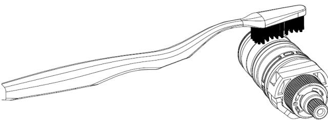
In case you need to clean the mesh filters use a toothbrush and rinse under running water, in the case of liming soak for 8-10 hours the cartridge in a solution of vinegar and water (50%) and then rinse under running water.
