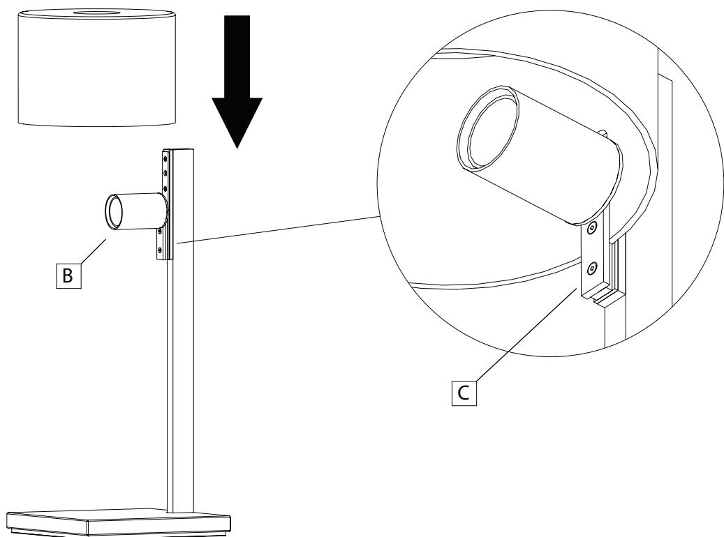
**EN** Install the glass diffuser between the lamp holder (B) and the plastic bracket (C).
