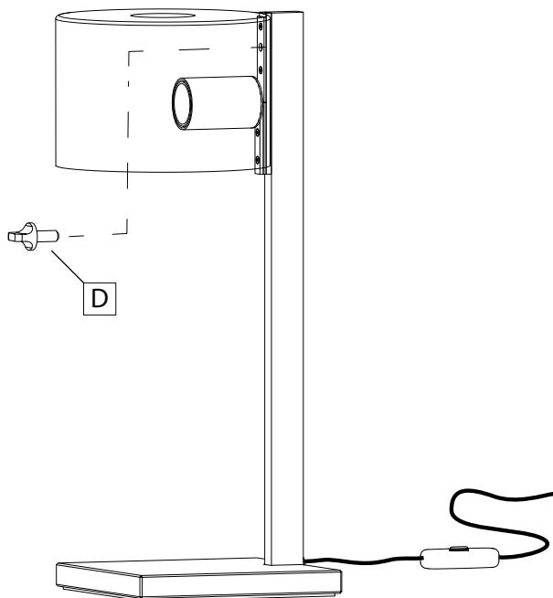
**EN** Fasten the plastic screw (D) to further secure the glass diffuser.
