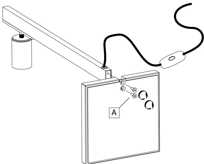
**EN** Attach the column to the base with screws (A).
