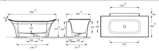
Product Specification: Semi-freestanding bath 180 x 90 cm. E6D158. Collection: GRANDS BOULEVARDS. DIMENSIONS: 180 x 90 cm. WEIGHT: 213 kg. MATERIAL: Neoroc. INSTALLATION TYPE: 39. VOLUME (L): 250/180. SHAPE: Rectangular. WASTE DIAMETER: 5.2. OPTIONAL: 2nd gel cushion.
